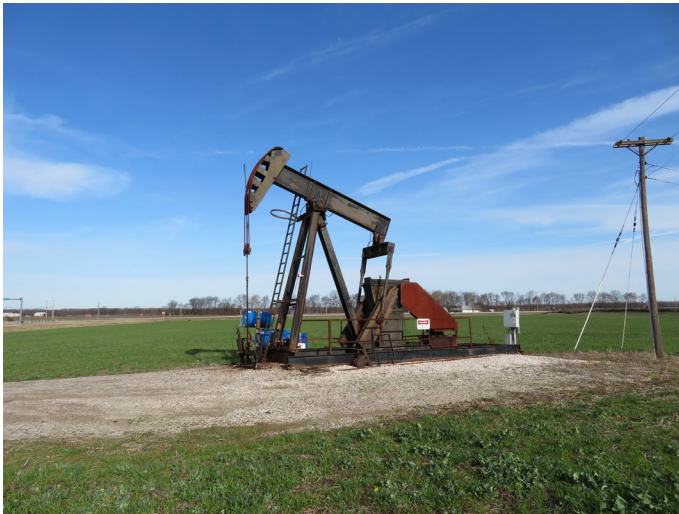
Figure 3.22-2: Typical Oil Well and Pumping Unit in Posey County
