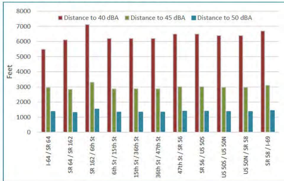
Figure 19. Estimated distances from Alternative P segments where traffic noise levels equal background levels.
